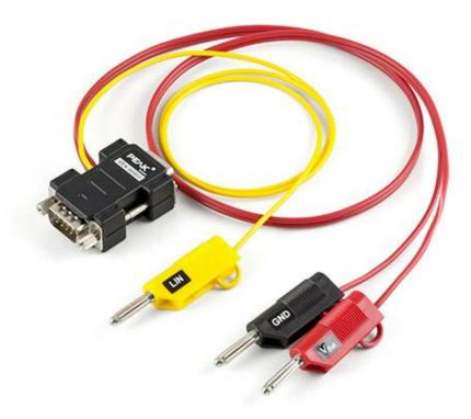
The PLIN-USB adapter is connected to the LIN bus via D -Sub. On the adapters PCAN-USB Pro FD and PCAN-USB Pro, the two field busses CAN and LIN are connected together via a D-Sub plug. However, a separate access to the LIN components is necessary.
