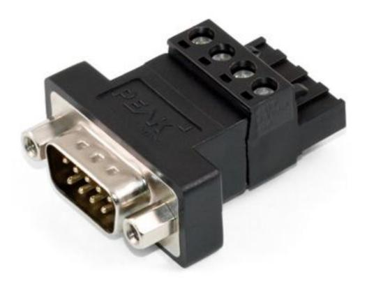
PEAK-System CAN hardware has a 4-pin screw terminal block as CAN connector for models in the DIN rail housing. The PCAN-D-Sub Connection Adapter provides a 9-pin D-Sub socket for the screw terminal pins. Thus, it is possible to plug in our standard CAN cable and to connect to our CAN PC interfaces.
